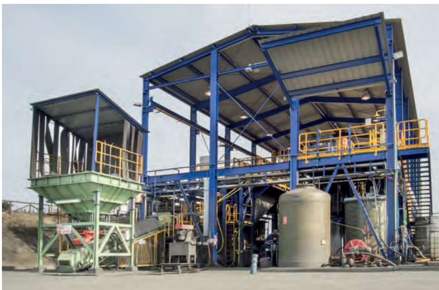
A 1 t/h pilot plant worked continuously for eight months over 2016/2017, treating 5,000 t of ore, to prove the new polymetallurgical process for the PMR project
